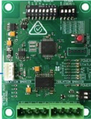
ICUNO-MOD (Located in the outdoor condenser)
